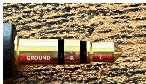
The virtual grounding of this included cable only works when the HAKUshin is switched on; hum noise may occur when the HAKUshin is switched off. Also, record playback when the battery is charging will reduce the level of hum noise reduction.
